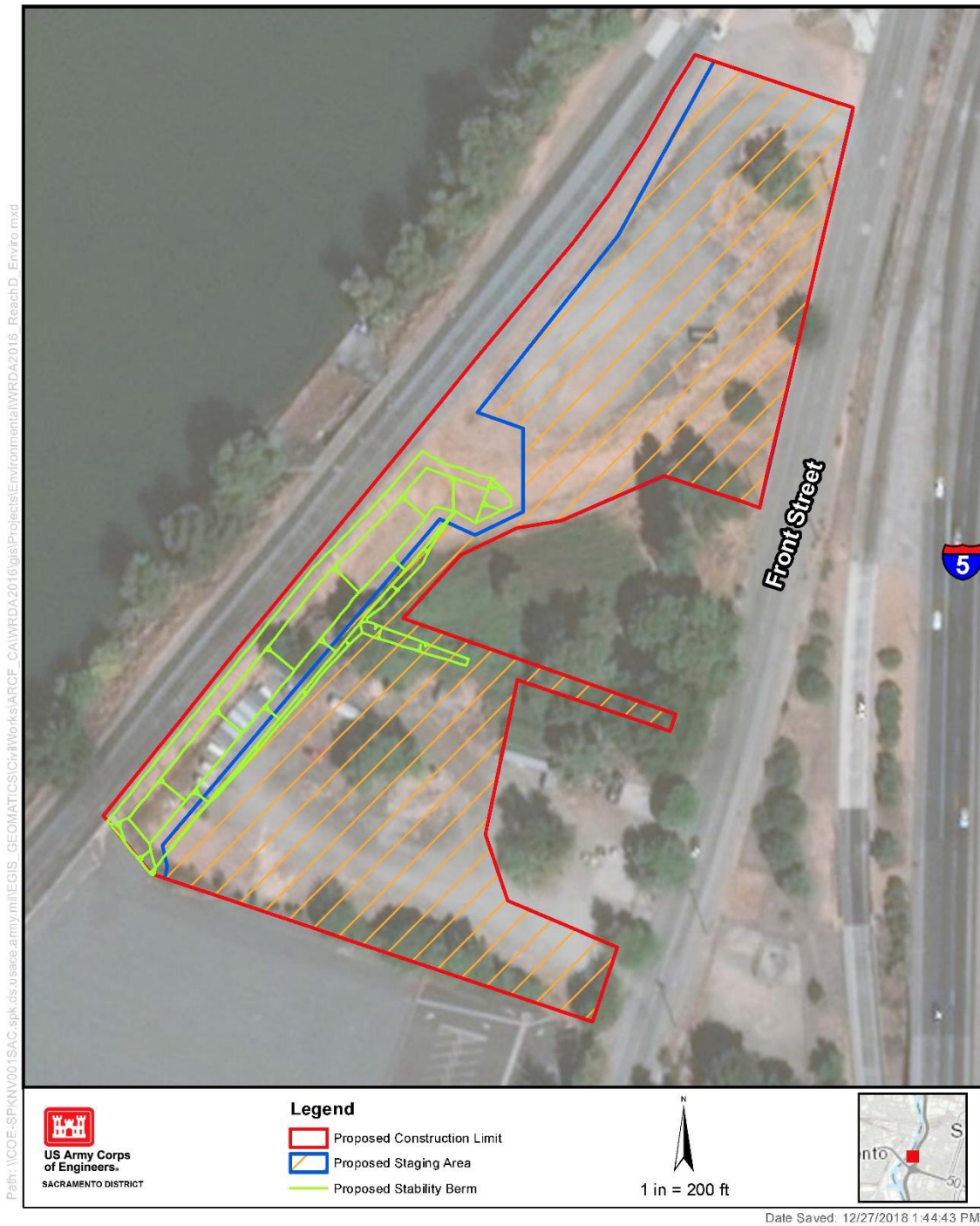
Figure 3. Alternative 2 – Drained Stability Berm Construction (Proposed Action).
