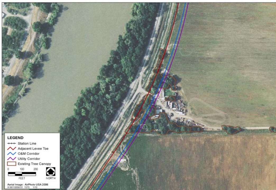
Figure1 - Example of Line Work Used to Calculate Woodland Impacts
